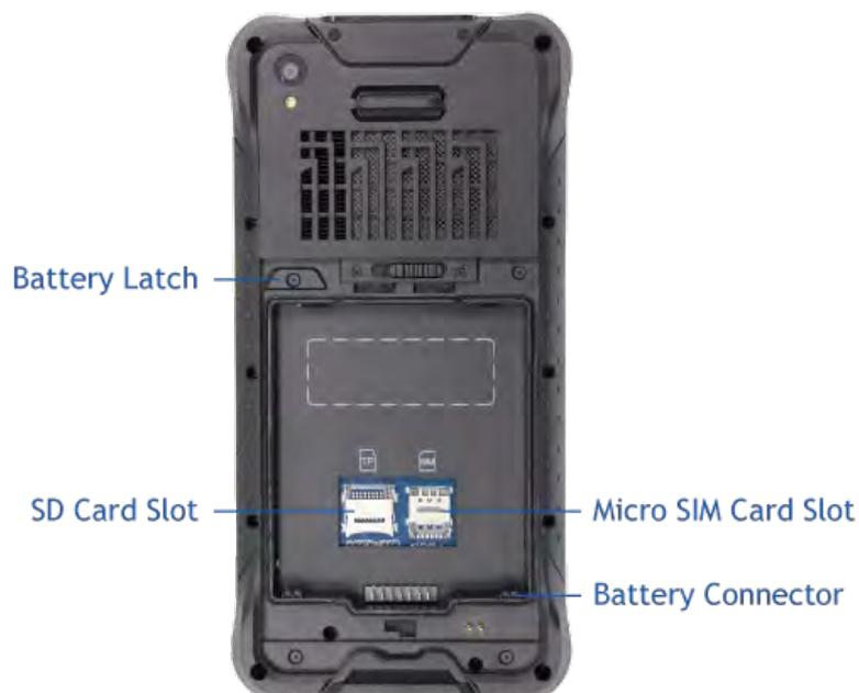
Step 2. After placing the SD card and SIM card into their designated slots, and the cards are enabled to use.
