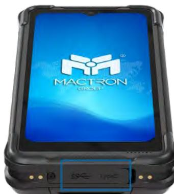
2. Insert the USB Type-C head of the power adapter into the USB Type-C port of the device.
