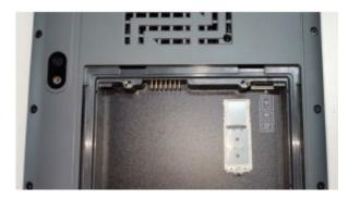
Step 2. After placing the TF card and Nano SIM card into their designated slots, reinsert the tray to enable use, as shown in the image below.
