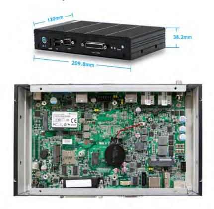
Equipped with onboard DDR4-2133 memory and M.2SSD storage, optional SATADOM, M2DOM, or SATA III, giving more flexibility for your solution deployment in any environments. Never have to worry about system stability whether the space is narrow, enclosed, or unstable condition. You know the system is reliable because everything is solidly build onboard without dangling cables inside.
